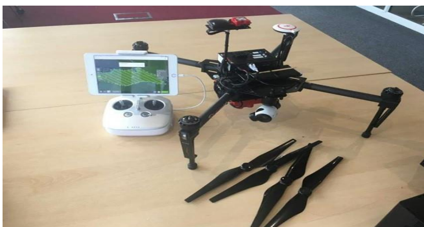
Figure 3.2: A drone with multispectral camera scans the grazing to measure biomass and feed values. Data is transmitted in real time by 5G.
